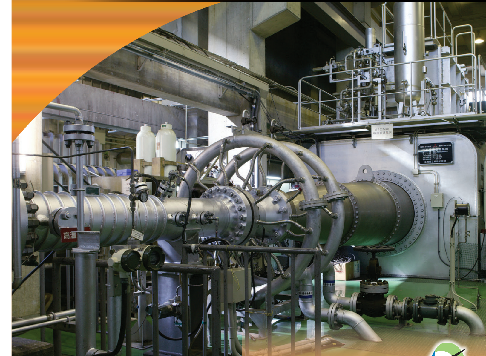
1.27m 極超音速風洞 1.27m Hypersonic Wind Tunnel
