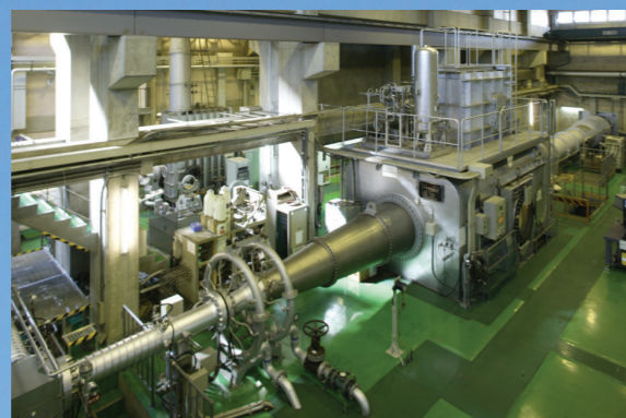
1.27m 極超音速風洞 1.27m Hypersonic Wind Tunnel
