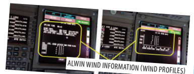
ALWIN wind information displayed on aircraft cockpit instruments (image provided by Japan Airlines Co., Ltd.)
