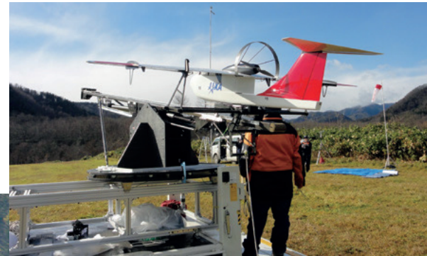
ABOVE: Disaster-monitoring unmanned aerial vehicle launch from a catapult mounted on a truck tray. LEFT: Flight testing of the disaster-monitoring unmanned aerial vehicle system using cameras to capture images from above a disaster site.
