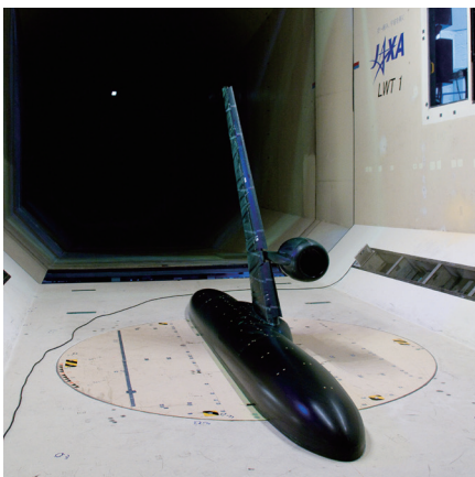
The 6.5 × 5.5 m low-speed wind tunnel has Japan's largest test section for aircraft and is capable of measuring large models.
