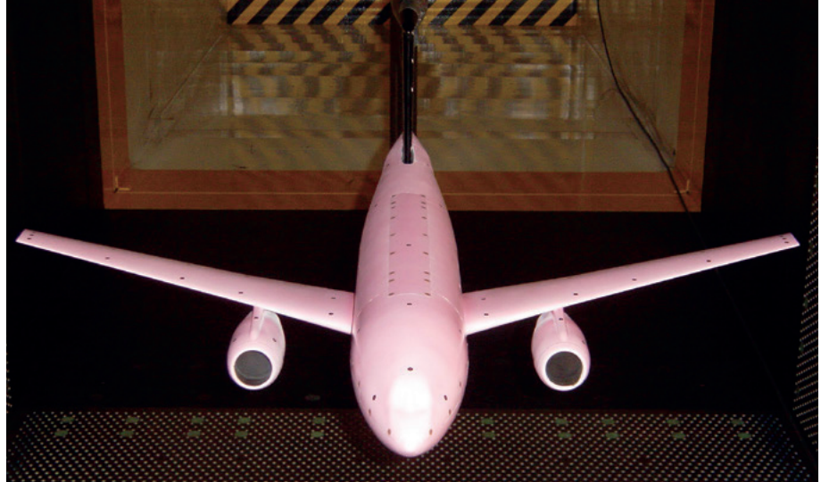
Pressure-sensitive paint (PSP) is light-emitting paint that changes brightness according to pressure. Pressure distribution is measured as an image, by measuring luminescent intensity from the PSP, using CCD cameras, etc. By coating PSP on a model, the pressure distribution for the entire surface can be measured. The redder the color, the higher the pressure - see below.
