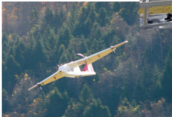
ABOVE: Disaster-monitoring unmanned aerial vehicle launch from a catapult mounted on a truck tray. LEFT: Flight testing of the disaster-monitoring unmanned aerial vehicle system using cameras to capture images from above a disaster site.
