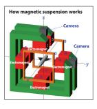
for the magnetic suspension wind tunnel is simple. When a current runs through the electromagnetic coils mounted to the sides, above, below, in front of and
