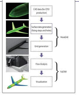
to be used for simulations of wind tunnel experiments.
