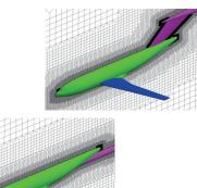
A model that incorporates supports into the calculations to simulate wind tunnel experimentation. An example showing conditions when the support goes through plates (top) and when the supports are attached directly (bottom)
