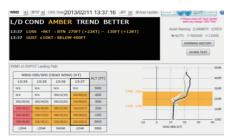
A screen shot of LOTAS that graphically visualizes wind information by assigning colors based on severity to aircraft operations.
