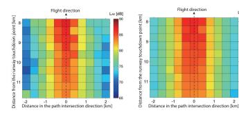
The measured aircraft noise (left) nearly matches the predicted value (right), proving high prediction accuracy. Deeper red colors correspond to higher noise levels.
