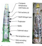
Cryogenic temperature test equipment loaded onto the sounding rocket
