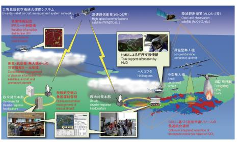
System configuration of the Integrated Aircraft Operation System for Disaster Relief (D-NET2)
