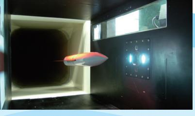
Suspending models in mid-air with magnetism enabled more realistic measurement
