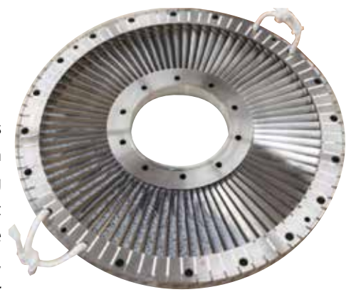
A low-pressure turbine prototype for flutter testing
