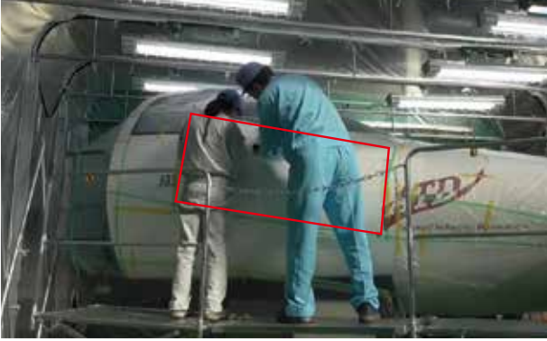
Applying a riblet coating to an actual-size aircraft mockup (joint research with Tokyo Metropolitan University; the red rectangle corresponds to the coating area)
