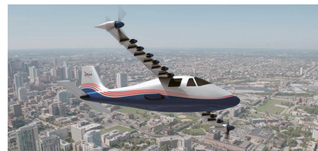
Concept image of X-57 Maxwell, NASA's all-electric X-plane (Image Credit: NASA Langley/Advanced Concepts Lab, AMA, Inc.)
