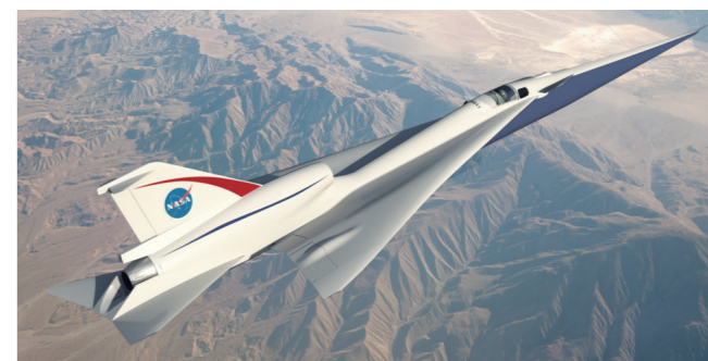
Concept image of NASA's supersonic X-plane, Quiet Supersonic Transport (QueSST) (Credit: NASA)
