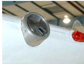
既存の機体電界計測センサの例 (field mill) https://archive.eol.ucar.edu/projects/t28/projects/chill-tex2002/
