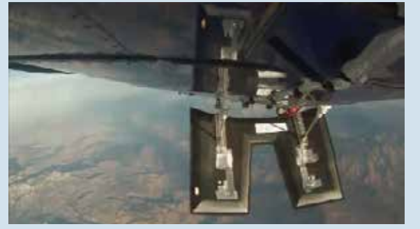
脱オートクレーブ成形法で作製した複合材製スピードブレーキの飛行実証試験 従来のアルミ合金製と同等の強度・機能で約40%の軽量化を実現 Flight demonstration test of a composite speed brake fabricated using out-of-autoclave curing methods. It is 40% lighter than a conventional aluminum alloy part, while having the same level of strength and functionality.
