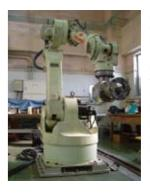
A model is supported from downstream by an industrial robot with six-degree freedom. Control of model position and attitude is easy and an efficient testing of flow field measurement around a model without moving measurement system is possible by moving the model. Aerodynamic force can be also measured by using internal six-component force balance.
