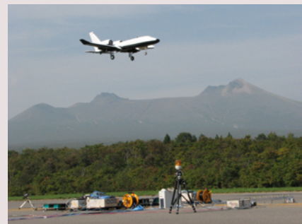
Noise source localization experiment with a model plane
