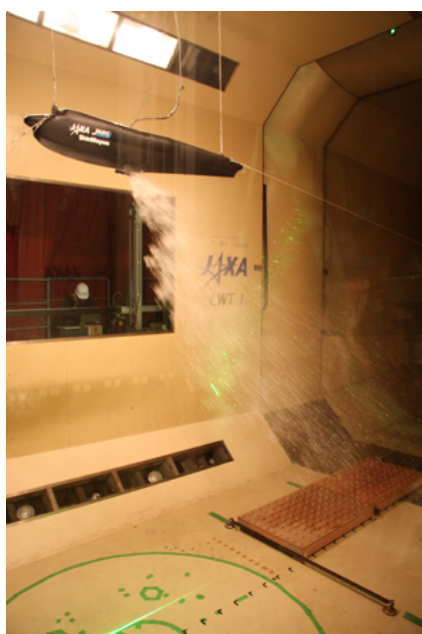
Fig.2 Water releasing test in a wind tunnel
