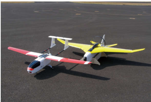
Fig. 2 Test model airplane to evaluate automatic flight techniques (left). Test model airplane to evaluate short-distance takeoff/recovery techniques (right).
