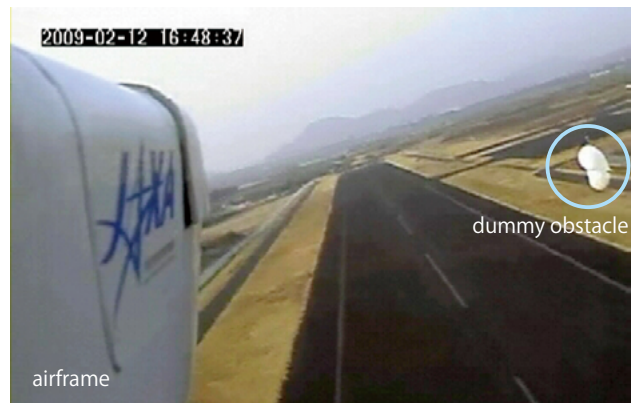
Fig. 4 Flight test to evaluate the obstacle-avoidance technique (image taken from the onboard camera)
