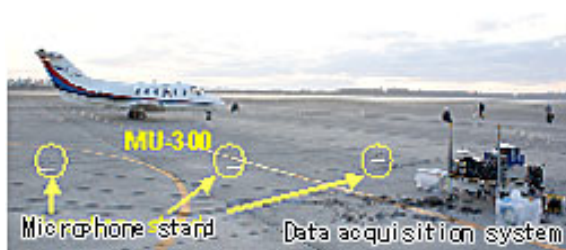
Fig.1: Ground engine-noise measurement test at Tokachi-Obihiro Airport
