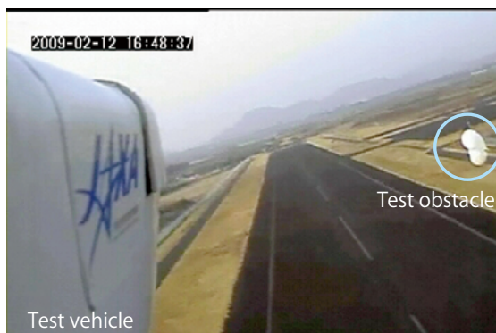
Fig. 2: Obstacle avoidance flight test
