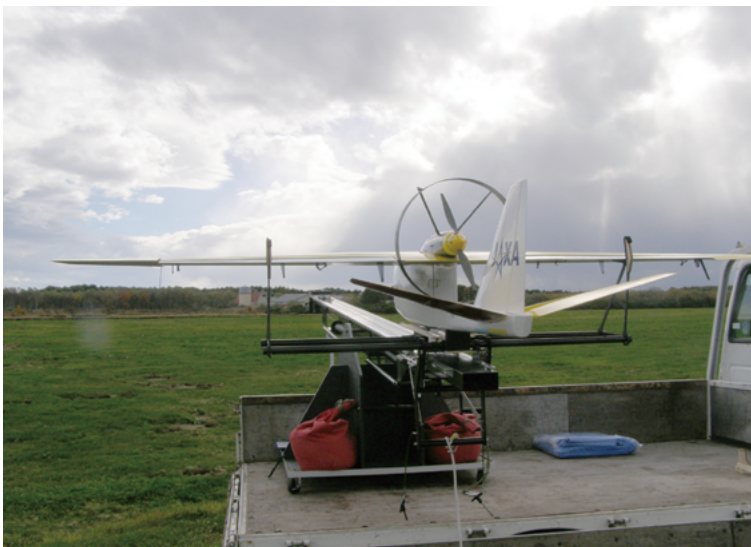
Fig.1: Test vehicle set on catapult launcher
