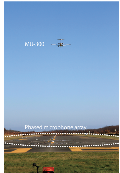
Fig.3: Business jet MU-300 flying over the phased array on the runway
