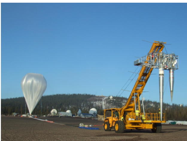
Preparing for launch. The test bodies are hanging from the crane. The low-boom model is on the left; the N-wave model is on the right.
