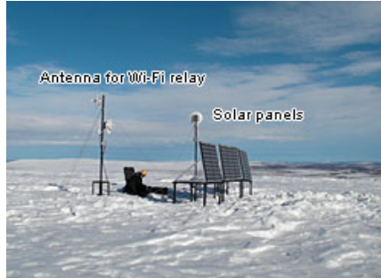
Relay points were set up in order to network the expansive area.
