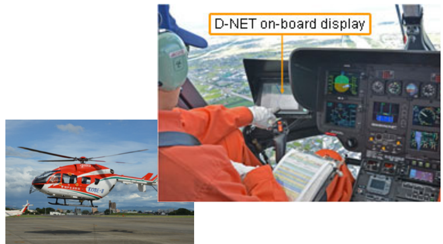
Fig. 4: Installation of D-NET on-board system
