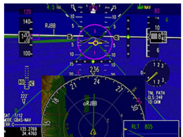
Fig.7: Test equipment showing the path transmitted from the ground with GLS
