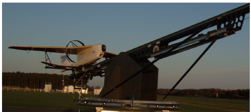
Fig.1 : Disaster-monitoring unmanned aerial vehicle (Right) On catapult launcher
