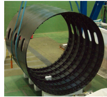
Structure of aircraft fuselage made with CFRP 3 m (diameter) × 3 m (length)
