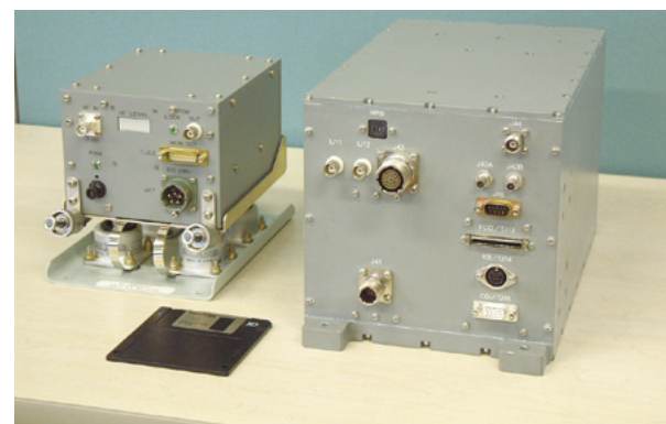
Fig. 1 ●“GAIA”, GPS-Aided Inertial navigation Avionics, developed by JAXA (for unmanned vehicles) Based on the GAIA technology, we are aiming at civil transport applications with this research and development.
