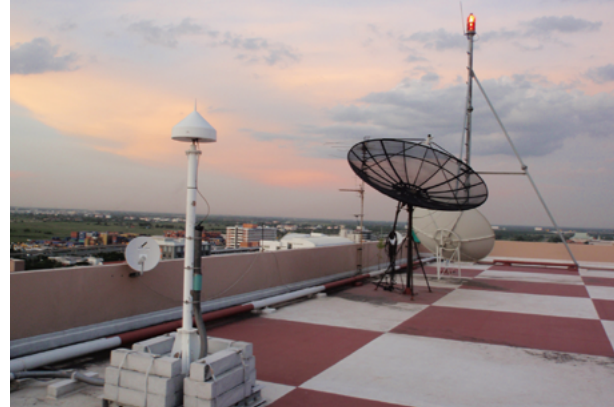
Fig.3 ●GPS ground station set up in Thailand (front left)
