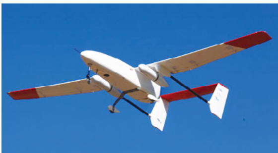
Existing JAXA fixed-wing sUAS (The sUAS for radiation monitoring will be developed based on this vehicle.)
