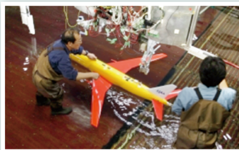
3. Set up in the suspension device. It is towed here at the start.
