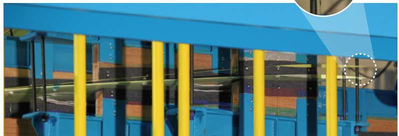
Fig.4 :Displacement of the wing tip in the maximum longitudinal fuselage and main wing bending case (composite photograph before and after loading)
