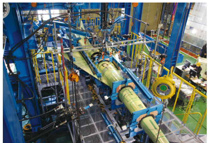
Fig.2: Configuration of the full-scale structural strength and stiffness evaluation test
