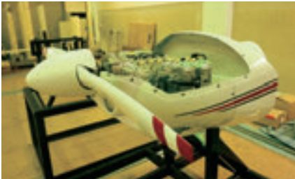
The propulsion system (electric motor system) developed by JAXA
