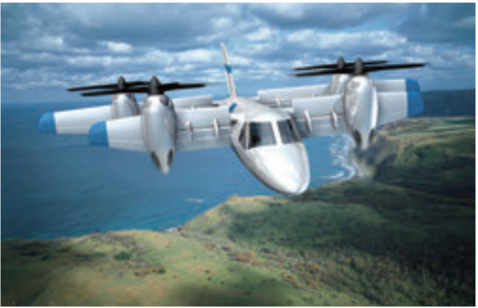
A four-engine tilt-wing VTOL business aircraft
