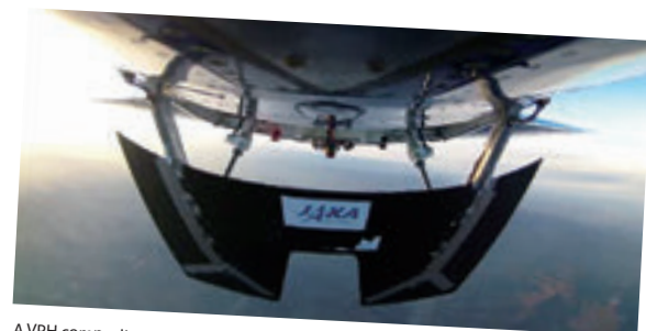
A VPH composite speed brake during flight testing
