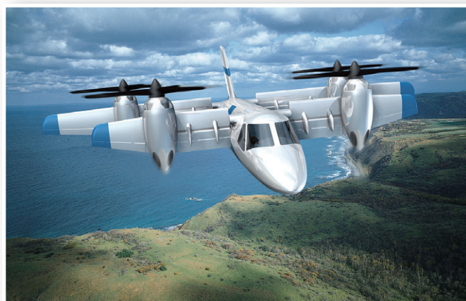
A four-engine tilt-wing VTOL business aircraft
