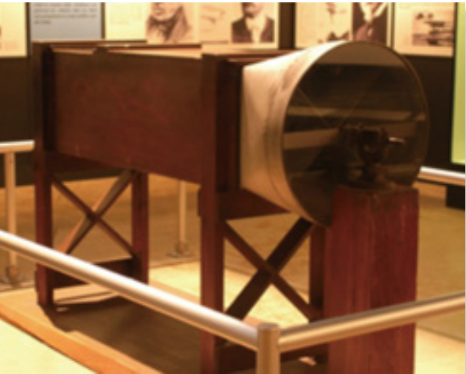
Replica wind tunnel device used by the Wright brothers. Image: U.S. Air Force.
