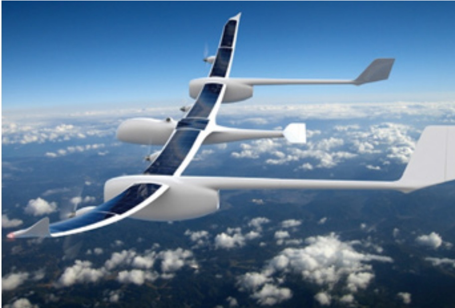
A conceptual image of the high-altitude long-endurance unmanned aircraft system that enables continuous observation for 72 hours.
