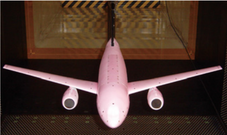
Pressure-sensitive paint (PSP) is light-emitting paint that changes brightness according to pressure. Pressure distribution is measured as an image, by measuring luminescent intensity from the PSP, using CCD cameras, etc. By coating PSP on a model, the pressure distribution for the entire surface can be measured. The redder the color, the higher the pressure - see below.
