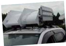
A car equipped with model Krueger flaps. It was preliminarily driven at the Tsukuba Space Center.
