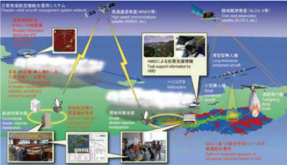
System configuration of the Integrated Aircraft Operation System for Disaster Relief (D-NET2)
