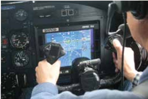
Flight tests of the curved approach with the MuPAL-a research aircraft
