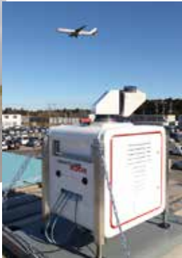
Measurements of wake turbulence using LIDAR around Narita International Airport
