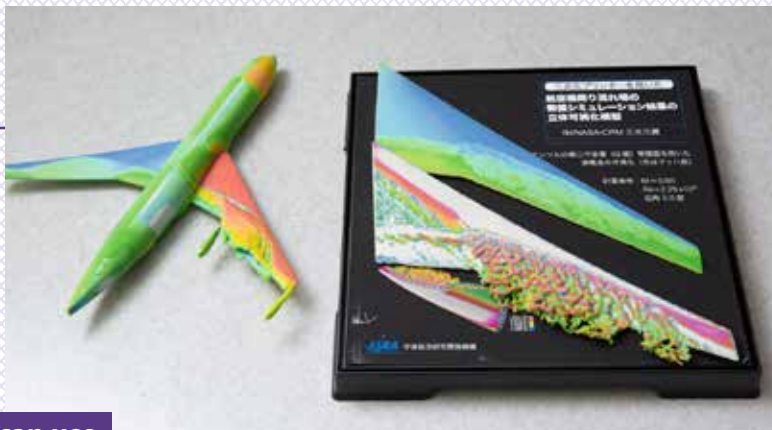
A 3D printer-based visualization of a numerical simulation of flow fields around an aircraft
