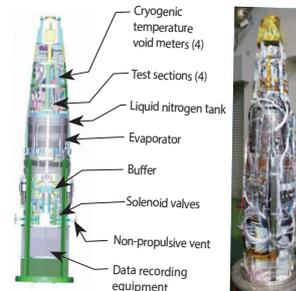
Cryogenic temperature test equipment loaded onto the sounding rocket
