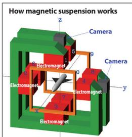
The mechanism for the magnetic suspension wind tunnel is simple. When a current runs through the electromagnetic coils mounted to the sides, above, below, in front of and
