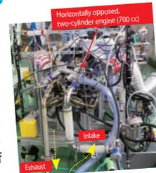
Equipment for testing high-altitude, turbocharged engines using a reciprocating engine
