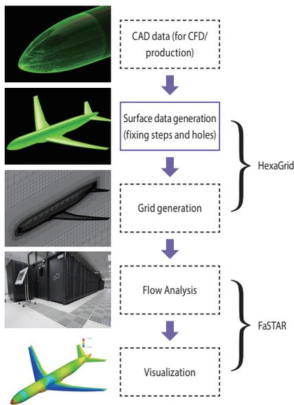
Calculations that used to take a whole day to complete with the code on the market are all done in less than an hour with FaSTAR—the fastest software of its kind in the world.
