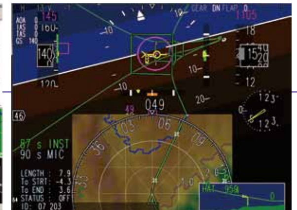
Tunnel-in-the-Sky displayed in cockpit
