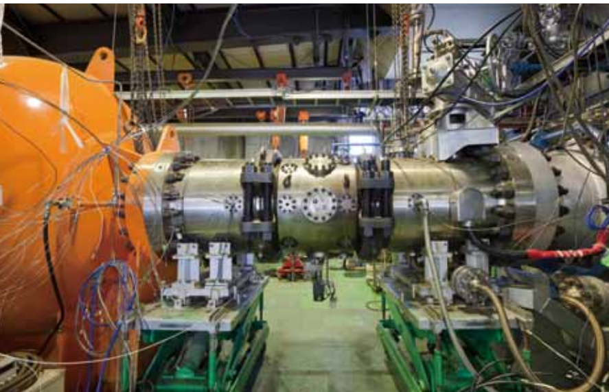
High-pressure and high-temperature combustion test facility The high-pressure and high-temperature combustion test facility tests partial models of jet engine combustors.
