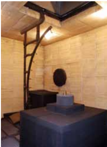
Noise test facilities Noise test facilities serve to determine noise sources, evaluate the effects of noise reduction devices, check noise propagation conditions, and perform other functions.
