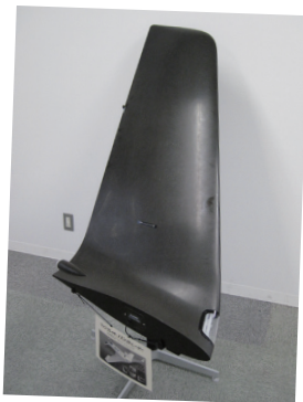
Life-size winglet model manufactured from recycled CFRP technology
