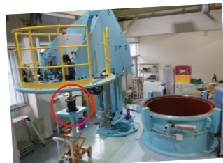
The large spin tester prior to an evaluation; the preparation process involves taking the lid (L) off the cylindrical vacuum chamber (R) and mounting the rotor (circled in red).
