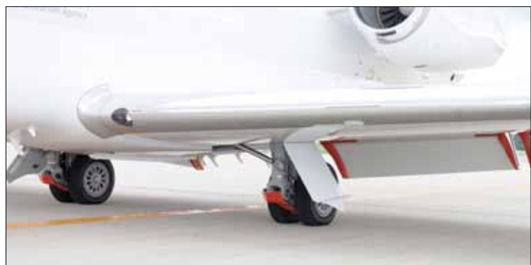
Flaps and landing gear of “Hisho” after modification for noise reduction. Modified locations are shown in red.
