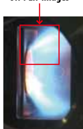
Combustion instability experiment at the high-temperature and high-pressure combustion test facility (Inlet pressure: 7 bar, Inlet temperature: 760 K). Time-series OH-PLIF images during a transition to combustion instability. The images were measured by the high-speed OH-PLIF at an interval of 1/10,000 of a second.
