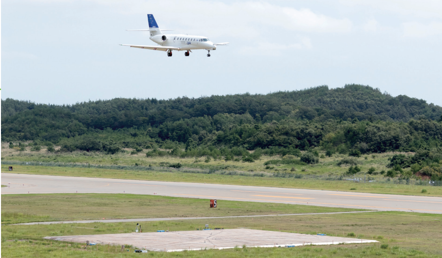
"Hisho" flies over the phased microphone array (see page 6) for measuring noise sources.
