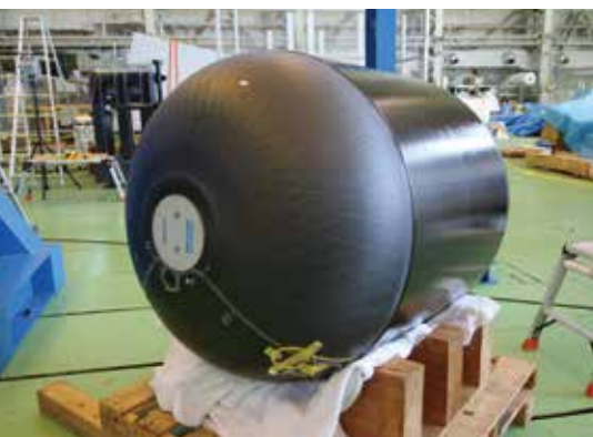
A prototype of a cryogenic tank for holding cryogenic liquid propellant
