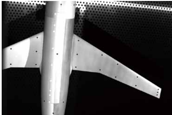
The small black spots on the model’s wings and fuselage are markers
