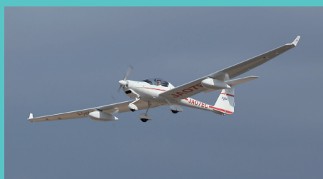
The electric motor-driven glider used for the FEATHER project
