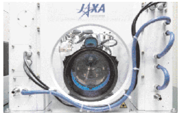
The developed turbulence detection system is light and compact enough for mounting on passenger aircraft
