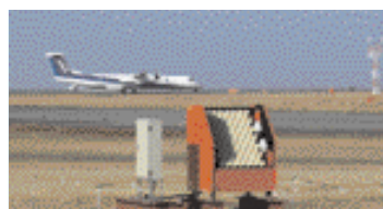
L: A SOLWIN Sodar (the red box in the middle-foreground area) in a trial setup at Oita Airport
