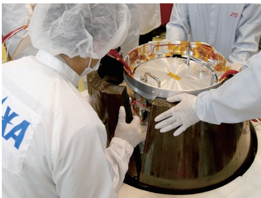
HTV Small Re-entry Capsule (HSRC) The HSRC, with a diameter of 84 cm, would be able to fit into the hatches of Kounotori (HTV) and the ISS.
