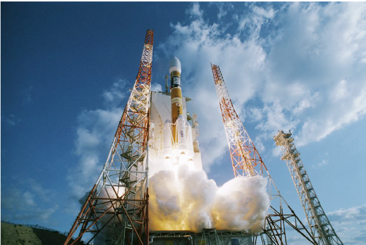
Fig. 1 Launch of the H-IIA rocket An artificial satellite loaded at the leading end of a rocket is launched into outer space. The satellite is covered with a fairing to avoid the effects of aerodynamic heating, etc. during flight in the atmosphere.
