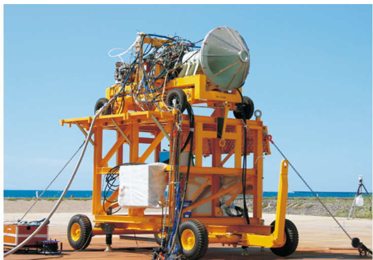
Fig.2 Scene from a noise-measuring test using YJ-69 engine at the Noshiro multipurpose test site in fiscal 2007
