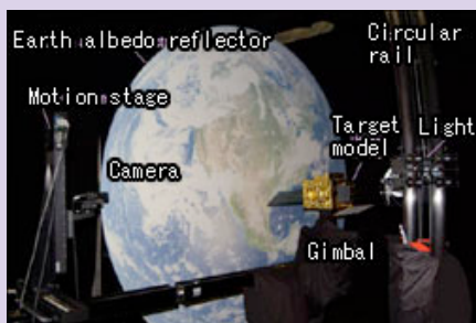
Experiment on the visual measurement technology for capturing debris
