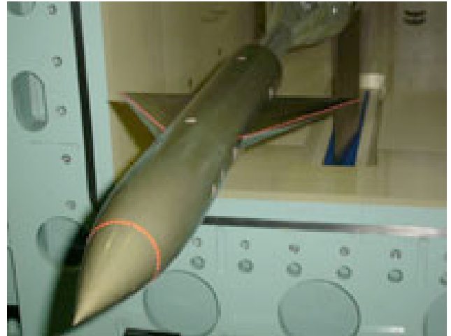
Fig.4 AGARD-B standard model installed in the JAXA supersonic wind tunnel
