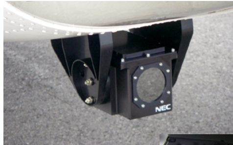
Fig.4 FLIR installed at the bottom of the airframe
