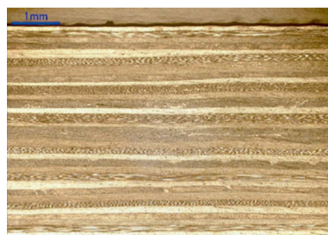
Fig.2 Polyimide-based CFRP (on the left) and microphotograph of its cross section (on the right)
