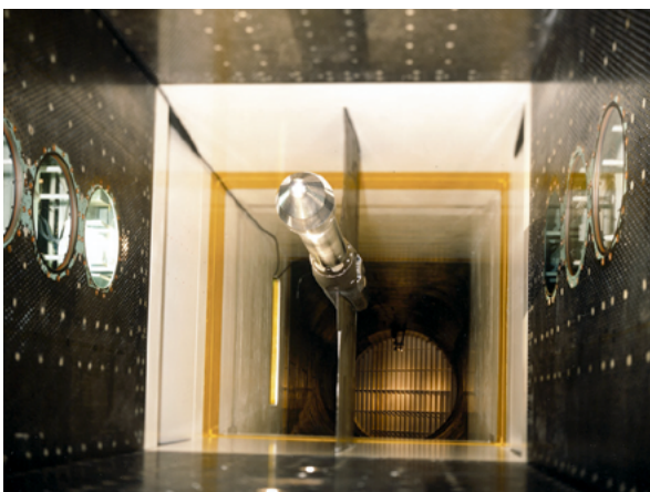
Fig.1: Performance assessment testing of the H-2 launch vehicle fairing
