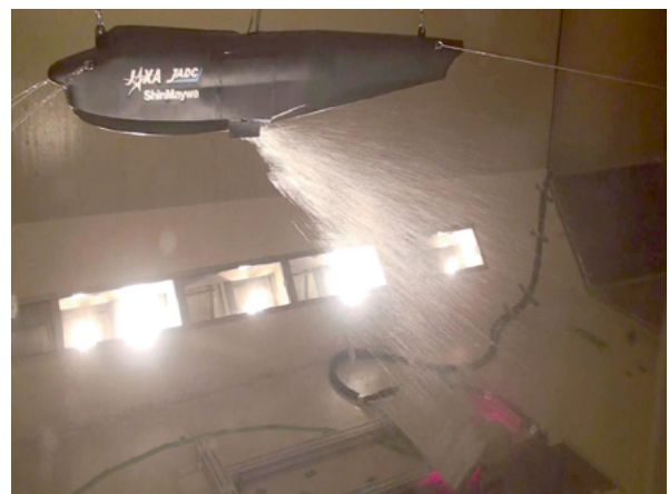
Fig.2 Water-drop testing of a firefighting amphibian
