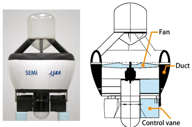
Fig.1 Ducted-fan flying robot
