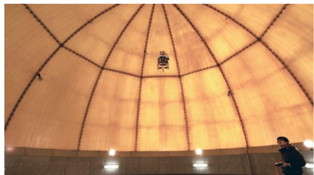
The initial flight test was conducted inside a dome allowing the transmission of GPS signals for control.
