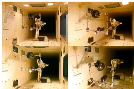
In order for a ducted-fan flying robot to ascend/descend, move forward/backward and left/right as well as fly freely in all directions at a low speed, it must be able to withstand airflow from various angles. Therefore, measurements were taken in a wide range of attack angles, from  $-90^{\circ}$  to  $+90^{\circ}$  .
