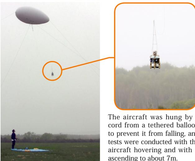
The aircraft was hung by a cord from a tethered balloon to prevent it from falling, and tests were conducted with the aircraft hovering and with it ascending to about 7m.
