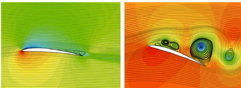
Even with a small angle of attack, separation is observed near the trailing edge of the wing.
