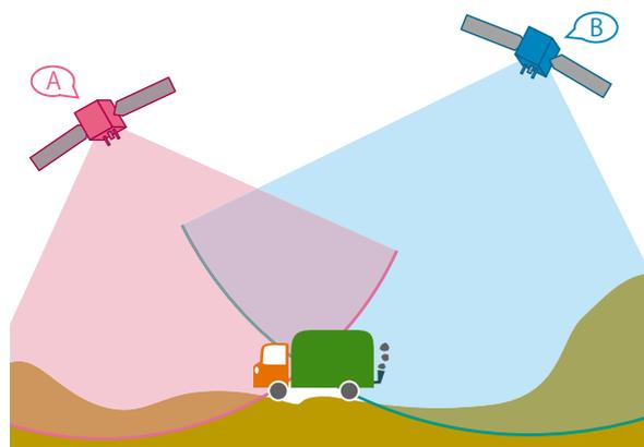
The radio waves emitted from satellite A at a specific time are received. The distance to satellite A can be determined as the product of the speed of the radio waves and the length of time for the radio waves to arrive after being emitted. By determining the distance to satellite B for the same time in the same way, the point where the distances intersect, in other words, your position, can be determined.
