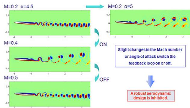
Fig. 5: Onset of the resonance phenomenon through acoustic feedback loop ( $Re=10,000$ )
