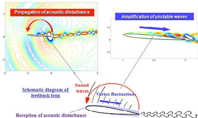
Fig. 4: Pressure field in a low-density flow around the wing ( $M = 0.2$ ,  $\alpha = 4.5$ ,  $Re = 10,000$ )
