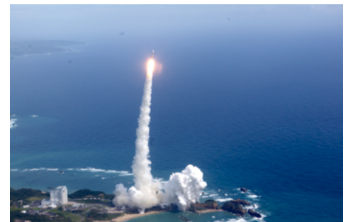
Flies into space with energy obtained by burning a mixture of liquid hydrogen and liquid oxygen.
