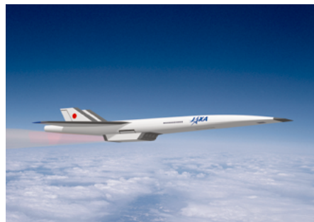
This aircraft, which has a total length of 90 m and seats for 100 people, crosses the Pacific Ocean in 2 hours.
