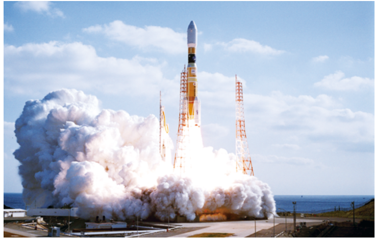
"Cargo", such as a satellite, is stored within the fairing at the tip of the launch vehicle.
