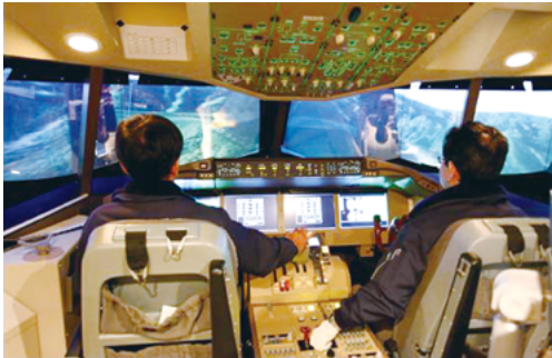
Fig.9: Verification of pilot support tool using the flight simulator
