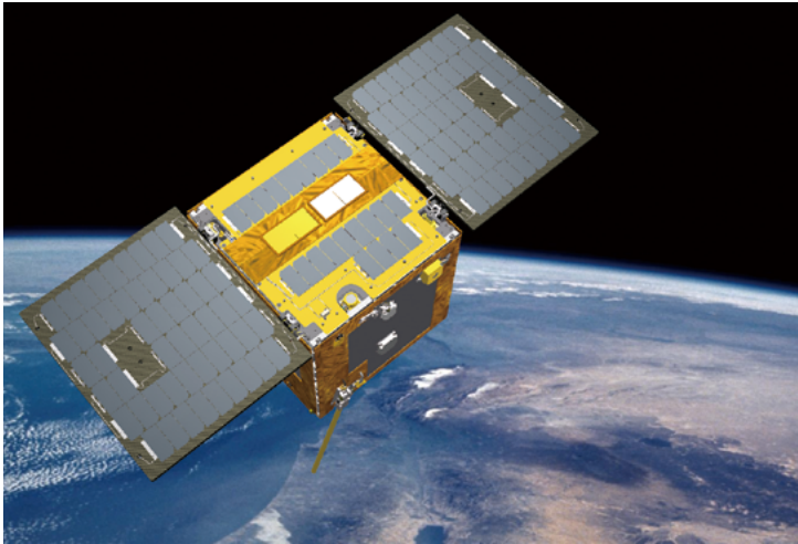
Fig. 1: Small demonstration satellite 4 “SDS-4” (illustration) inserted at an altitude of 677 km
