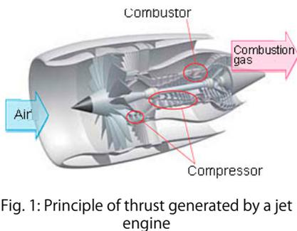
Fig. 1: Principle of thrust generated by a jet engine
