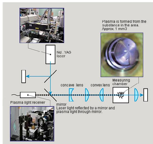
Laser light travels to reflectors and through lenses, and is condensed at an area in the measuring chamber. Due to the strong energy of the laser, atoms separate from the molecules of the substance in that area, and then atoms and electrons separate to form plasma (excited state). Immediately afterward, the atoms emit light (plasma light), then return to the ground state. The emitted plasma light passes through lenses via the plasma light receiver to be spectroscopically measured.
