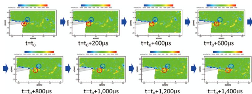
The downstream flow of the vortex created at the top surface of the model’s wing (shown by the blue arrow) and the vortex created at the bottom surface (shown by the red arrow) could be captured.
