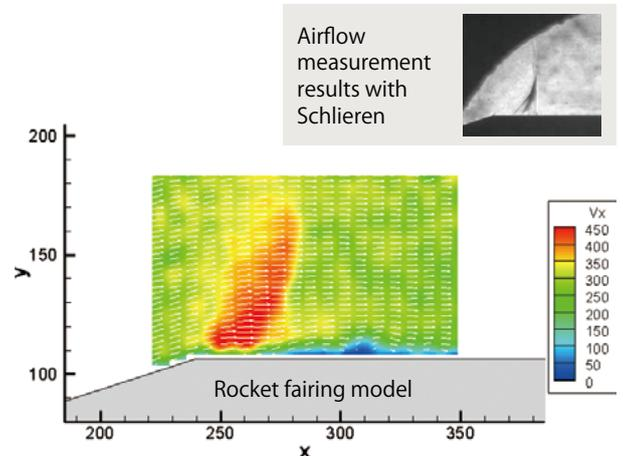
We succeeded in capturing a shock wave that occurred on the model, similar to that with the Schlieren visualization method performed in the past.
