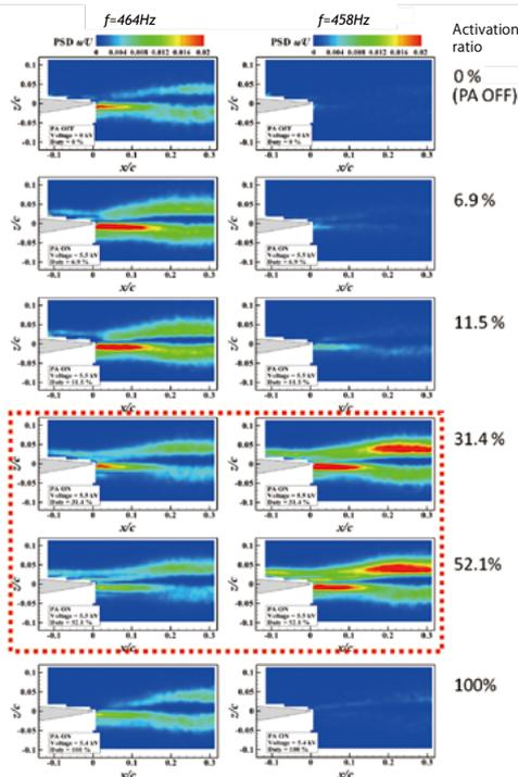
By activating plasma actuators, the change in velocity for a 464 Hz sound is reduced. However, it was revealed that the change in velocity for a 458 Hz sound increased by activating the actuators to 31.4% and 52.1%. This shows a good correlation to the actual occurrence of noise.
