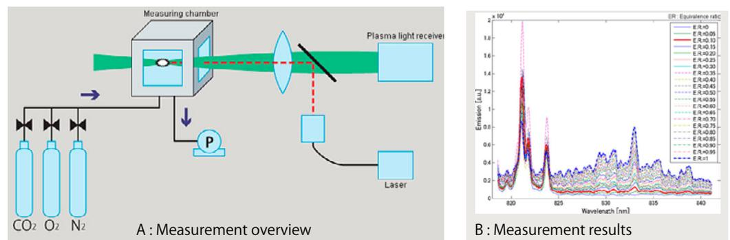
Fig. 3: LIPS test for establishing the equivalence ratio calculation method under high temperature and high pressure
