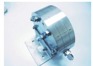
C: Membrane gas-liquid separator
