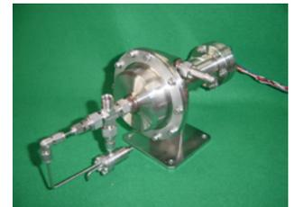
A: Rotating gas-liquid separator
