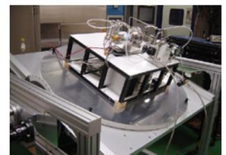
Fig. 3: Test of rotating gas-liquid separator with a test stand in the direction of the gravitational force
