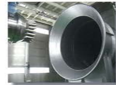
排気ダクト (Exhaust Collector & Augmentor Duct)
