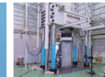
CFRP panel compression test
